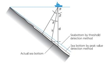
Angle of inclination  $\theta = 30^{\circ}$  Direction angle of transducer  $\beta = 3^{\circ}$
